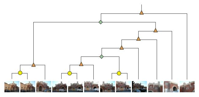
Figure 3: An example of a dendrogram for a 12 image set. The circle  $\circ$  corresponds to the creation of a stereo-model, the triangle  $\triangle$  corresponds to a resection-intersection, the diamond  $\diamond$  corresponds to a fusion of two partial independent models.
