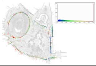
Figure 15: Results of point cloud comparison between laser and SAMANTHA for "Brà" and "Duomo di Pisa". The colour of the SAMANTHA's point cloud encodes the residual distance, consistently with the histogram shown in the insert (this figure is best viewed in colour). Units are in meters.
