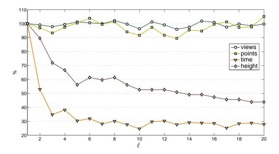
Figure 5: This plot shows the number of reconstructed tie-points, images, height of the tree and computing time as a function of the parameter  $\ell$  in the balancing heuristics. The values on the ordinate are in percentage, where the baseline case  $\ell=1$ .
