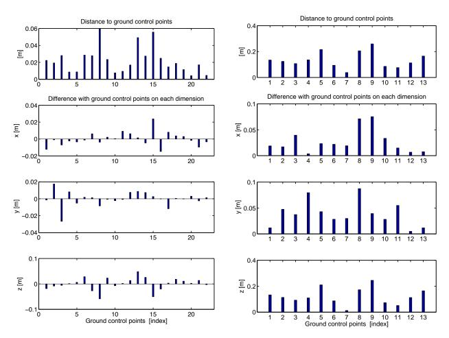
Figure 11: Top: Distance of computed 3D points to ground control points for the "Ventimiglia" image-set. Bottom: Differences on each dimension (X-Y-Z).
