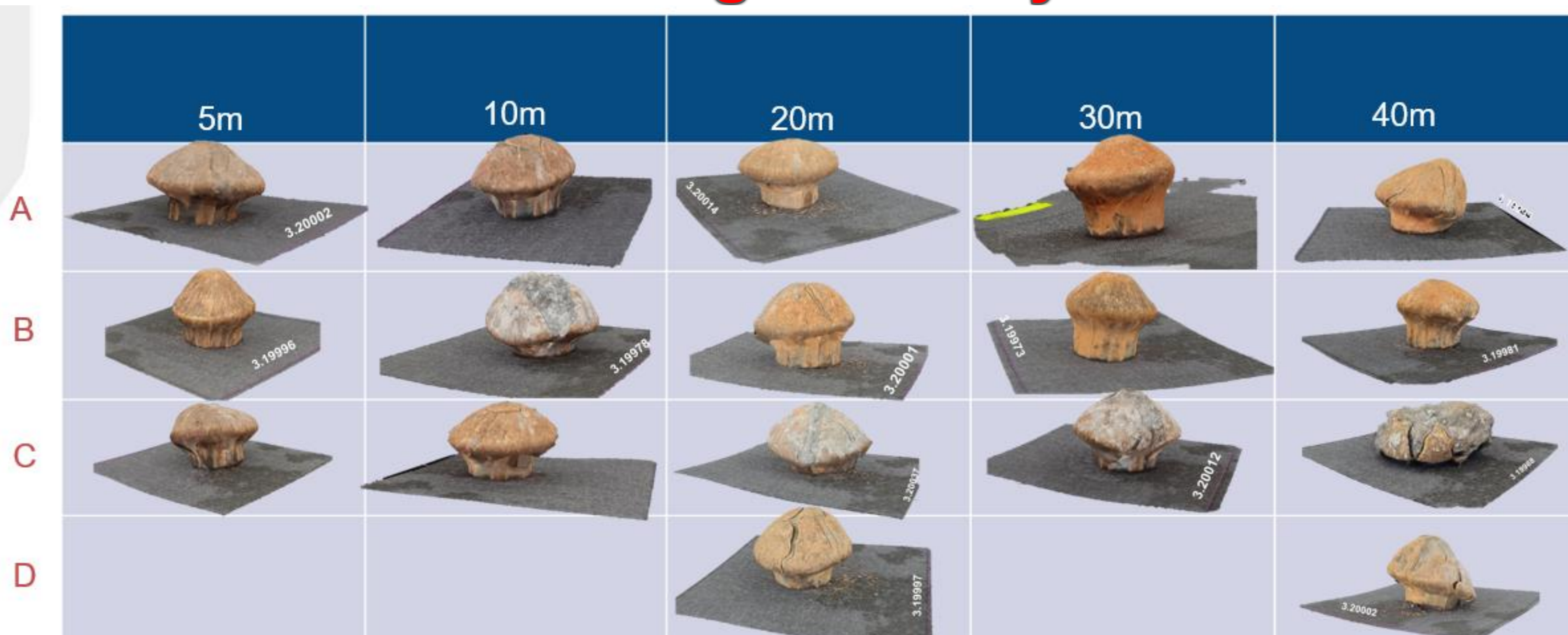
Figure 1. Photogrammetry of 9mm Luger shots against clay brick. No deformation was calculated for projectiles after hitting steel plates targets due fragmentation.
